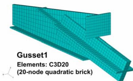
Fig. 11 Finite element mesh of Gusset 1
