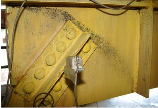
Fig. 4. (a) Out-of-plane buckling of the gusset plate
