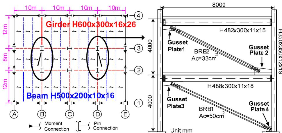
Fig. 8 Floor framing plan and BRBF elevation
