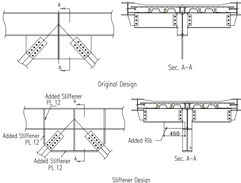
Fig. 3 (a) Original design of the gusset plate and (b) Details of added stiffeners
