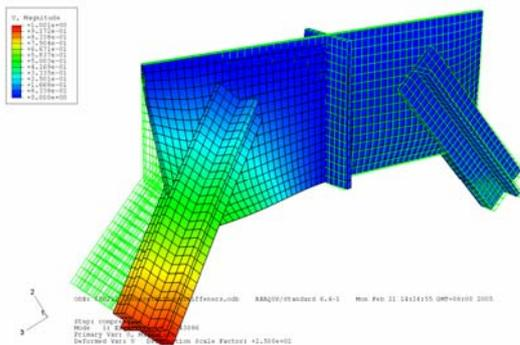
Fig. 7 (a) FE Model of un-stiffened gusset plate
