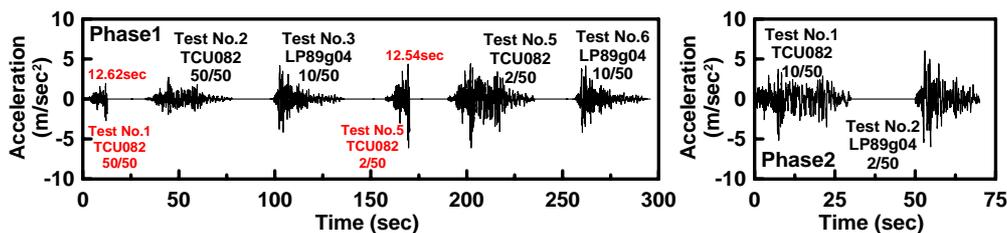
Fig. 2 Ground acceleration time history in PDTs
